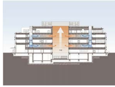
Natural ventilation system
