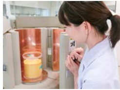
2. Setting the radioactive material measuring instrument
