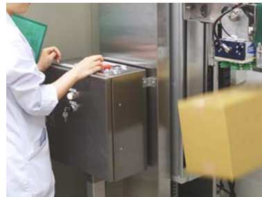
Products are drop-tested from heights equivalent to those encountered during freight-handling and shelf-stocking to assess them for deformation and breakage.
