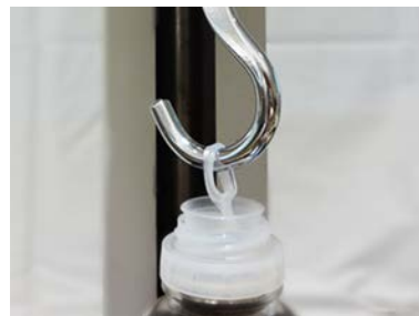
Removing a pull tab from dressing container to assess ease of opening.
