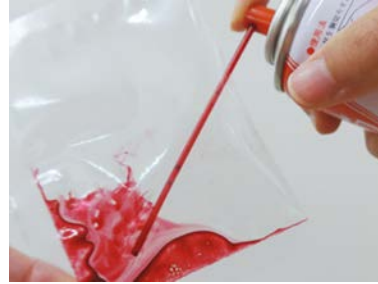
We use red penetrant to check for minute seal defects and ensure containers seal properly.
