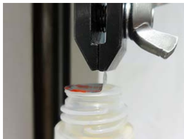
Assessing foil seal on Mayonnaise container for ease of removal.
