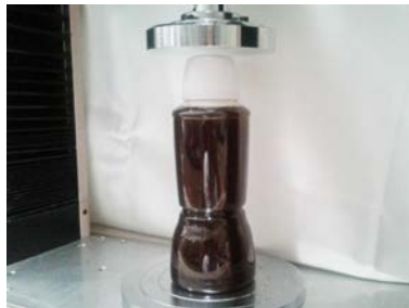
Containers are pressurized to assess the load they are capable of withstanding.
