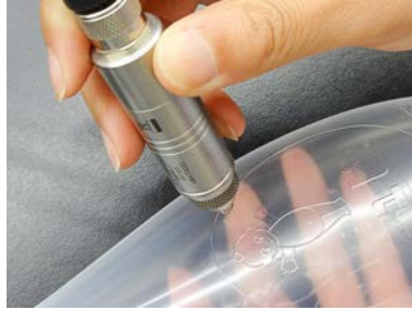
Container thickness is measured precisely to assess whether it is sufficient to preserve quality and consistent across all portions.
